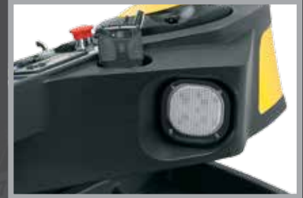
LED work light with ultrasonic sensor
